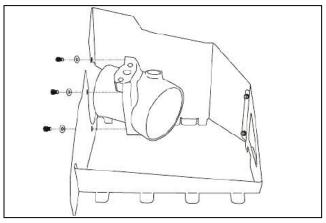
**6.** Assemble the air filter adapter to the cool air dam using the (3) ½-20 bolts and washers provided.
