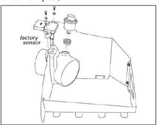
7. Fasten the factory sensor on top of the Airaid adapter using the (2) 8/32 screws and washers & a 3/32 Allen Wrench to tighten. In addition, mount the factory rubber grommet and filter minder onto the Airaid plastic adapter.
