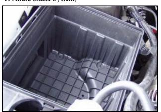
**4.** Loosen the clamp connecting the factory air box lid to the factory air intake tube and unclip the factory air box lid and remove entire filter/intake assembly from vehicle. (Note: leave the lower factory air box lid in place)
