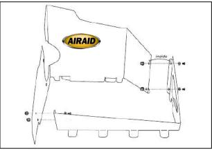
**5.** Assemble Airaid Quick Fit cool air dam panels using the (4) 6/32 bolts, washers and nuts provided. Apply the Airaid Foil Decal onto the Panel as
