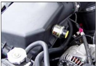
**2.** Remove the factory filter minder with grommet and retain for use with the Airaid Intake System.
