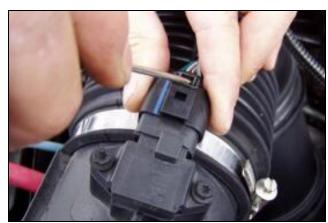
**9.** Re-connect the wire harness to the sensor on top of the adapter.
