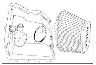
**10.** Mount Airaid Premium Filter to the filter adapter and tighten hose clamp. Next, press the weather strip onto the top of the Cool Air Dam (Hint: start at a corner and work toward the edges).
